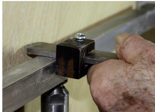
This long tool rest can also be useful for turning long spindles and the same principle makes it easy to make a perfectly parallel spindle or a length with a uniform taper.
